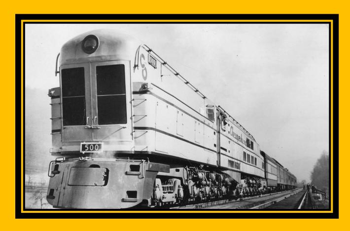
Westinghouse-Baldwin "Blue Goose" gas turbine. Built 1950, 4,000HP.
